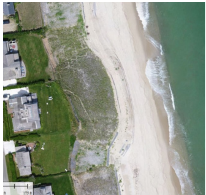
Aerial view of the bluff and the geotubes holding the bluff from erosion
